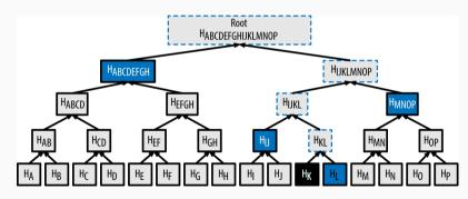
A node can prove that transaction *K* is included in the block by producing a Merkle path, which consists of 4 hashes:  $H_L$ ,  $H_{IJ}$ ,  $H_{MNOP} \in H_{ABCDEFGH}$ . Only  $\log_2(N)$  32-byte hashes needed
